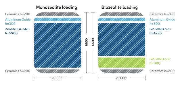
Given all of the possible deviations in adsorbent operation (variations in stock composition, changes in adsorbent load, etc.), on the basis of simulation and experience in the use of sorbents in similar systems, we can offer different load options.
