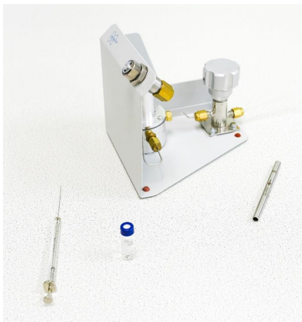
Figure 1 – Loading the calibration standard into the Tenax® TA tube using an injection unit for TD tubes.
