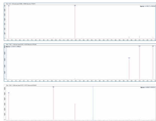
Mix of brizant explosives. Chromatogram and spectra obtained in SIM mode for better selectivity and sensitivity. 1 – Trinitrotoluene (TNT) 2 – Hexogen (RDX) 3 – Pentaerythritol tetranitrate (PETN)
