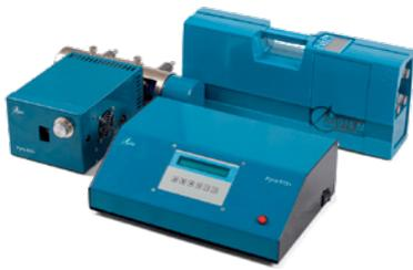
RA-915M mercury analyzer with PYRO-915+ attachment
