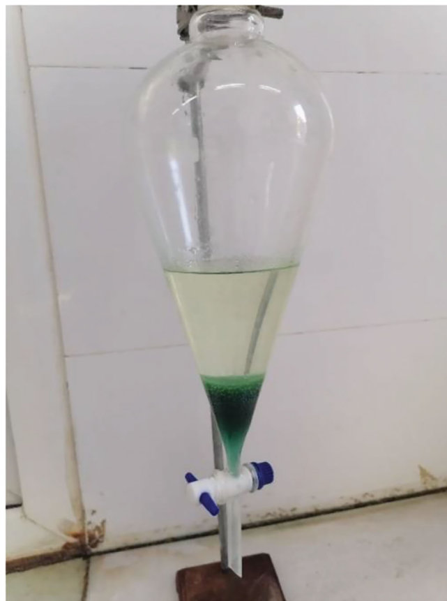
FIGURE 4 Two-phase liquid after the catalytic oxidation process.
